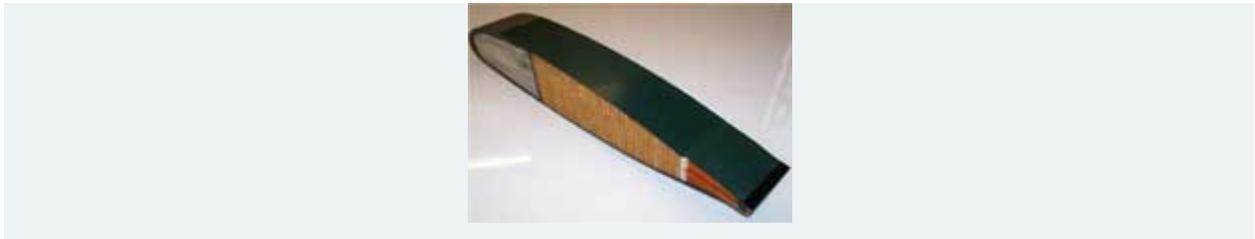
A prototype morphing helicopter rotor blade. A similar device could help improve wind turbines. Credit: Paul Weaver et al.
